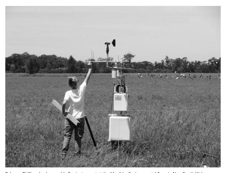
Rebecca Phillips checks an eddy flux instrument at the Manildra Environmental Farm in New South Wales, Australia, as part of a research project seeking to determine how much carbon emissions are captured through managed grazing. She's now heading a similar project in North Dakota.
