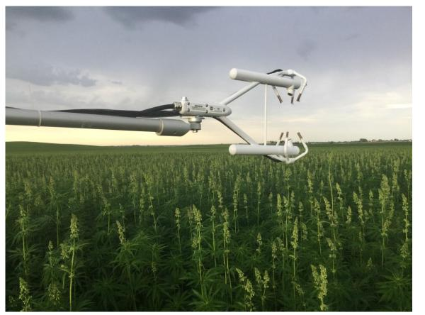
Net ecosystem production Precipitation Sensible heat flux Latent heat flux Incoming solar radiation Photosynthetically active radiation Soil heat flux Soil moisture and temperature Air temperature Relative humidity
